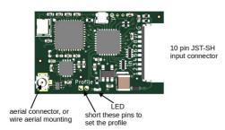
The MT01b on-board LED is repeated to an external LED via the JST-SH 6p, pin 3. This will need a series LED appropriate to the LED current and required brightness. A 1K ohm resistor is used on Micron transmitters - see one of the wiring diagrams below for an example LED connection. The on-board LED is switched off after 60 seconds.
